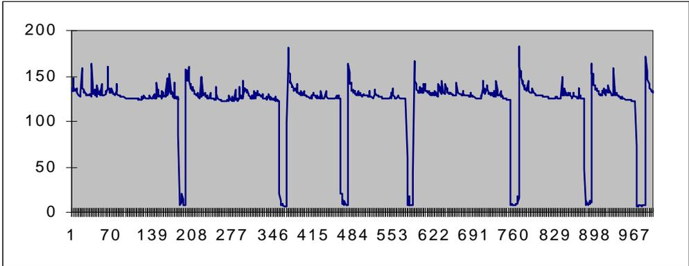
Graph 2: Watts used for each 10 minute interval during the monitoring of a poorly functioning older refrigerator
