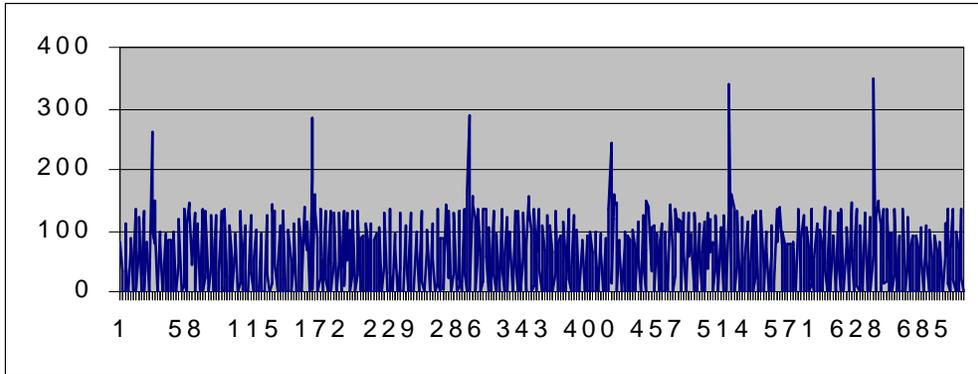
Graph 3: Watts used for each 10 minute time interval during the monitoring of a new energy efficient refrigerator
