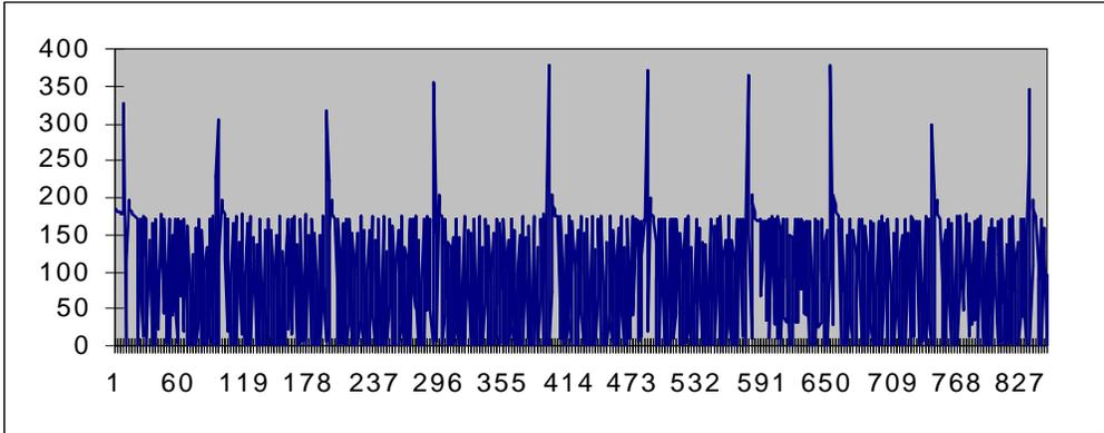
Graph 1: Watts used for each 10 minute time interval during the monitoring of a properly functioning older refrigerator
