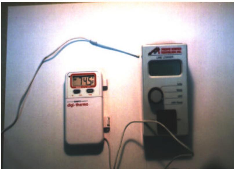
Picture 3: Inexpensive Digital Thermometer and PST Line Logger
